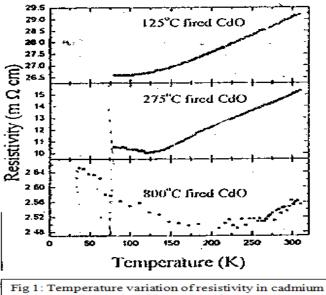
oxide samples produced by 36 hour heat treatment at the indicated temperatures. Difference in the resistivity scale implies very low resistivity for the 800°C fired sample
